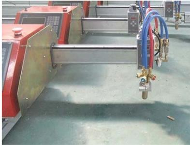
◆If metal sheets are rugged, should use THC to adjust distance from torch to metal surface.
