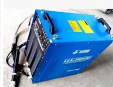
Our plasma can cut 0.3-30mm; our oxygen can cut 5-150mm
